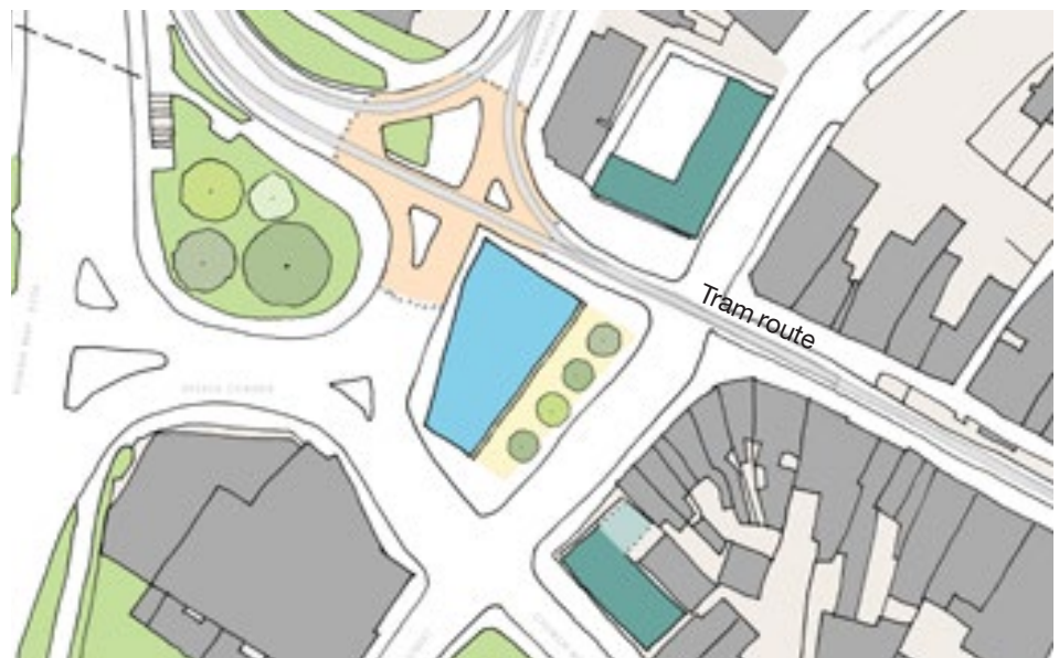
Figure 42: Indicative diagram showing possible improvements to the Reeves Island site without changing traffic flows. New homes with active ground floor uses on the western side would create usable public space or gardens on a widened footway (see page 138 for key).
