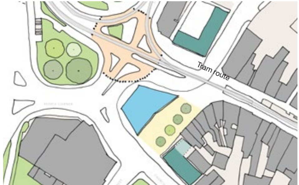
Figure 41: Indicative design for 'Peninsularising' Reeves Corner. This would create an open space enclosed by buildings, and improve the quality of the direct pedestrian link between North End and Minster Quarter. The building on the 'peninsularised' site would be more accessible and traffic flows would be rationalised.
