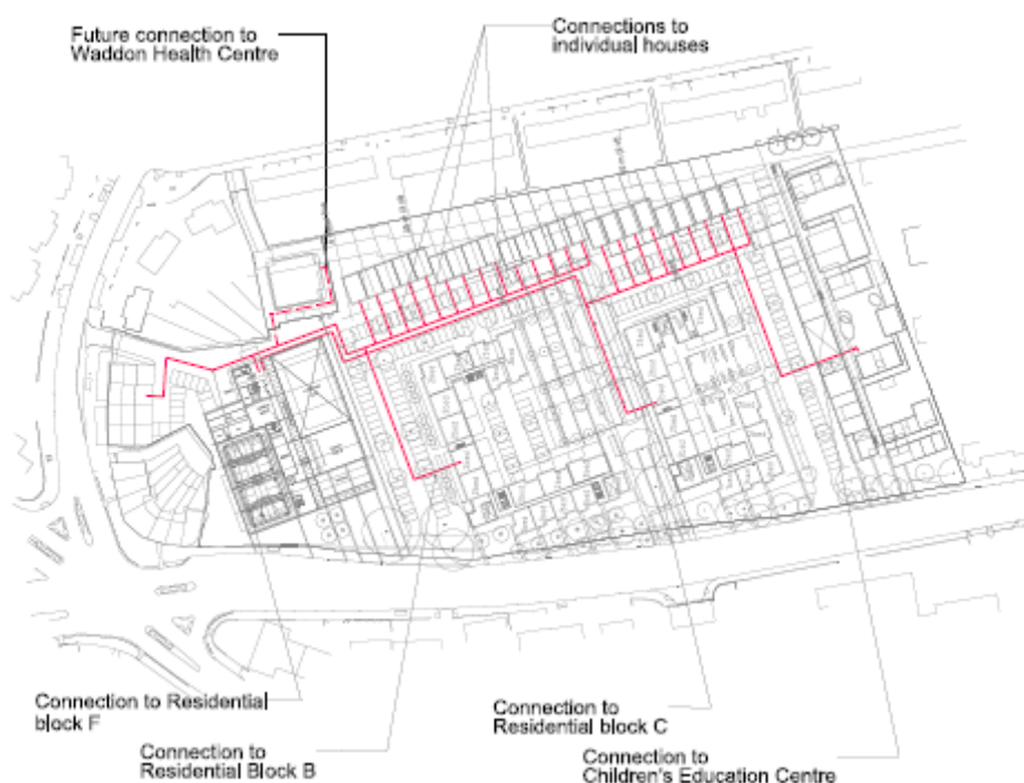
Figure 34: Proposed heat network for the Waylands site (Source: Levitt Bernstein)
