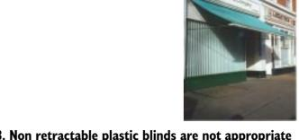
fig. 13. Non retractable plastic blinds are not appropriate as they permanently obscure parts of the shopfront and introduce discordant materials and shapes into the street scene, particularly in historic areas
