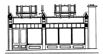
fig. 6. Large, internally illuminated box fascias should be avoided. The fascia size should be related to the overall proportions of the building. As shown in the diagram above
