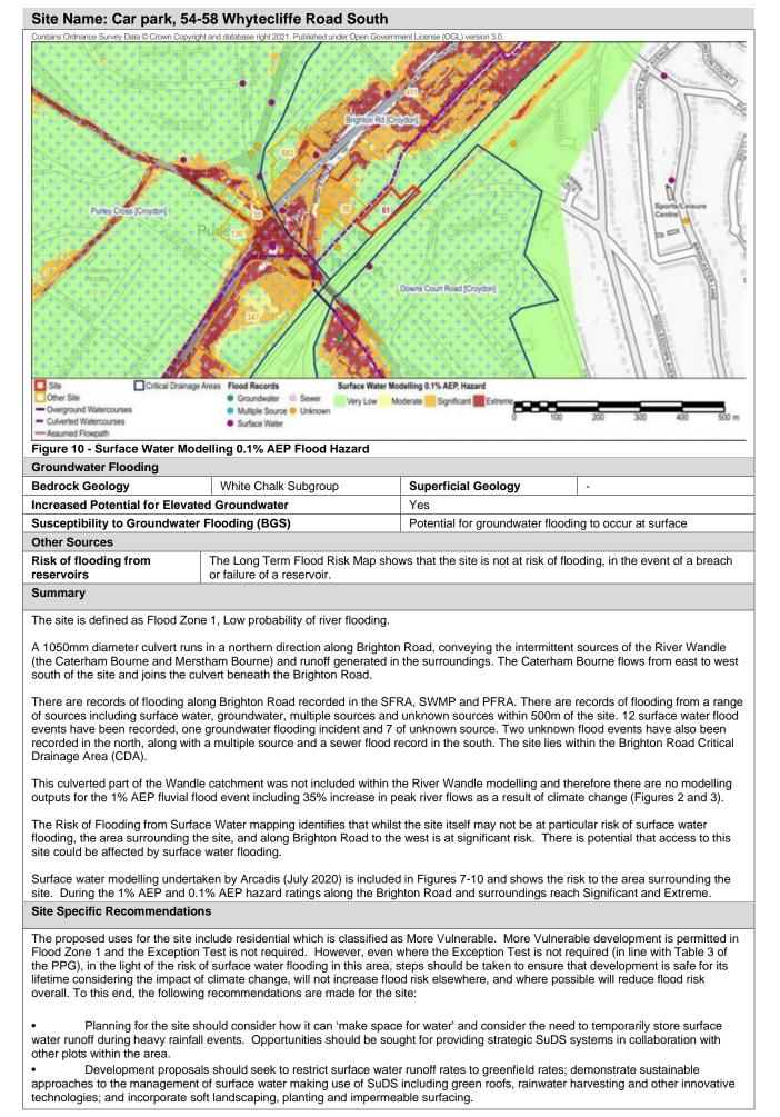
• Finished floor levels for More Vulnerable development should be set 600mm above ground levels. Where surface water modelling is available, finished floor levels should be set above the modelled flood level for the 1% AEP event, including a 300mm freeboard. Flood depths for the modelled 1% AEP event are shown in Figure 7.
